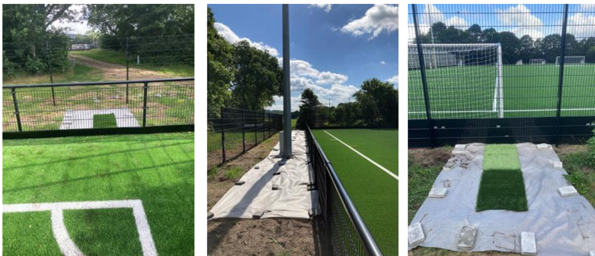
Figure 3: Sampling pads for granulate discharge over fences and barriers
