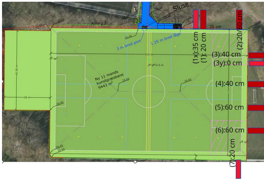
Figure 5: Illustration of Silkeborgbanen, with sampling positions and fence-heights
