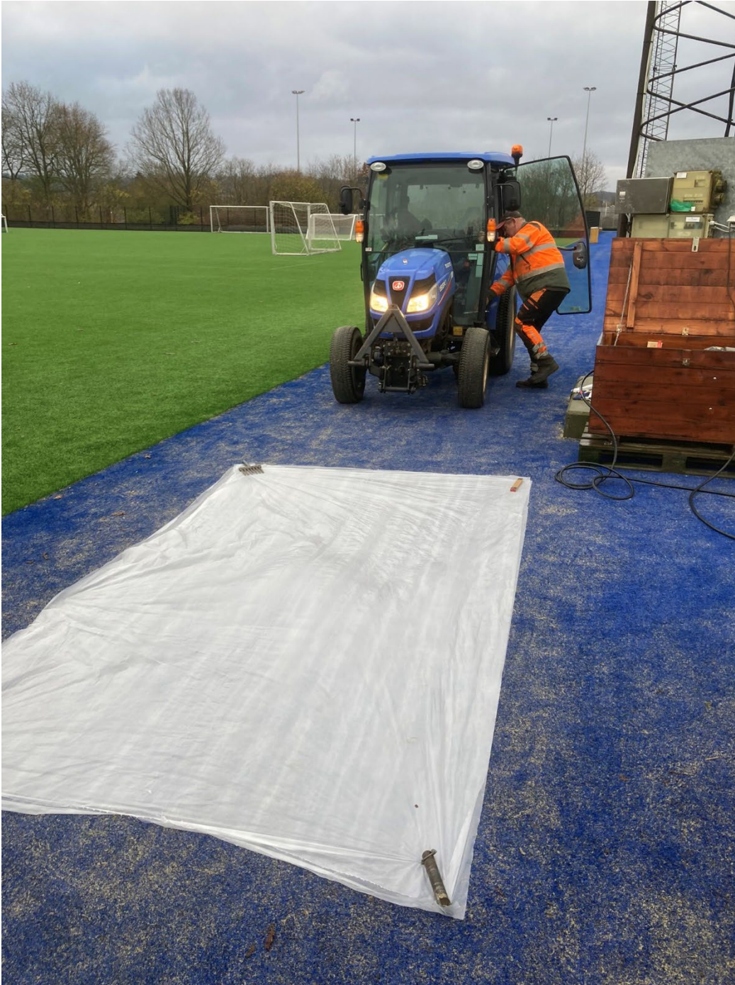
Figure 11: Sampling from tractor used for maintenance operations was done by thoroughly cleaning the machine while collecting infill material on a plastic sheet.
