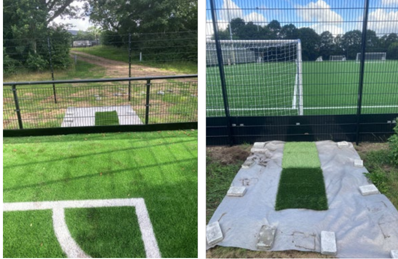
Figure 4: Sampling pads for granulate emitted over fences and barriers.
